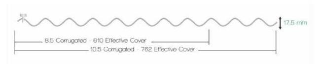
Corrugated sheeting is the traditional and familiar S-Rib profile for roofing and cladding applications. It is the oldest and most commonly used roofing profile because of its easy handling and fixing properties and related strength. The S-rib is derived from sinus curve and offers very strong and structural properties.
